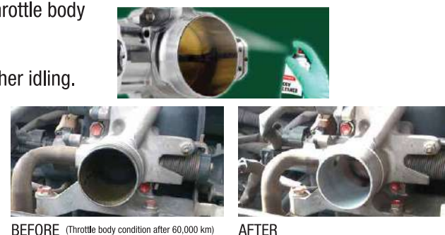
BEFORE (Throttle body condition after 60,000 km)
